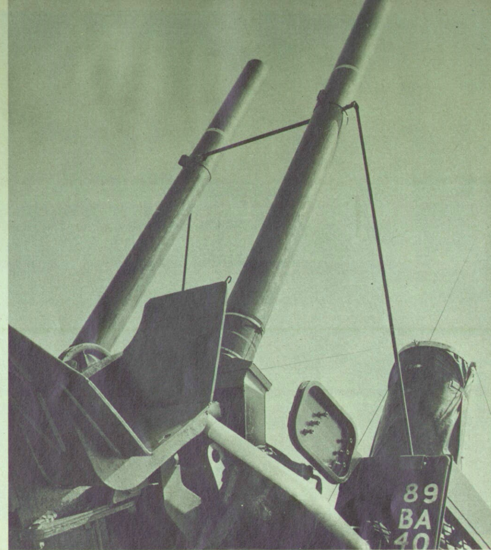
Above: Development work on snorkels by the branch now enables beach armoured recovery vehicles to be effectively used for work in water depths of twelve to fifteen feet.
