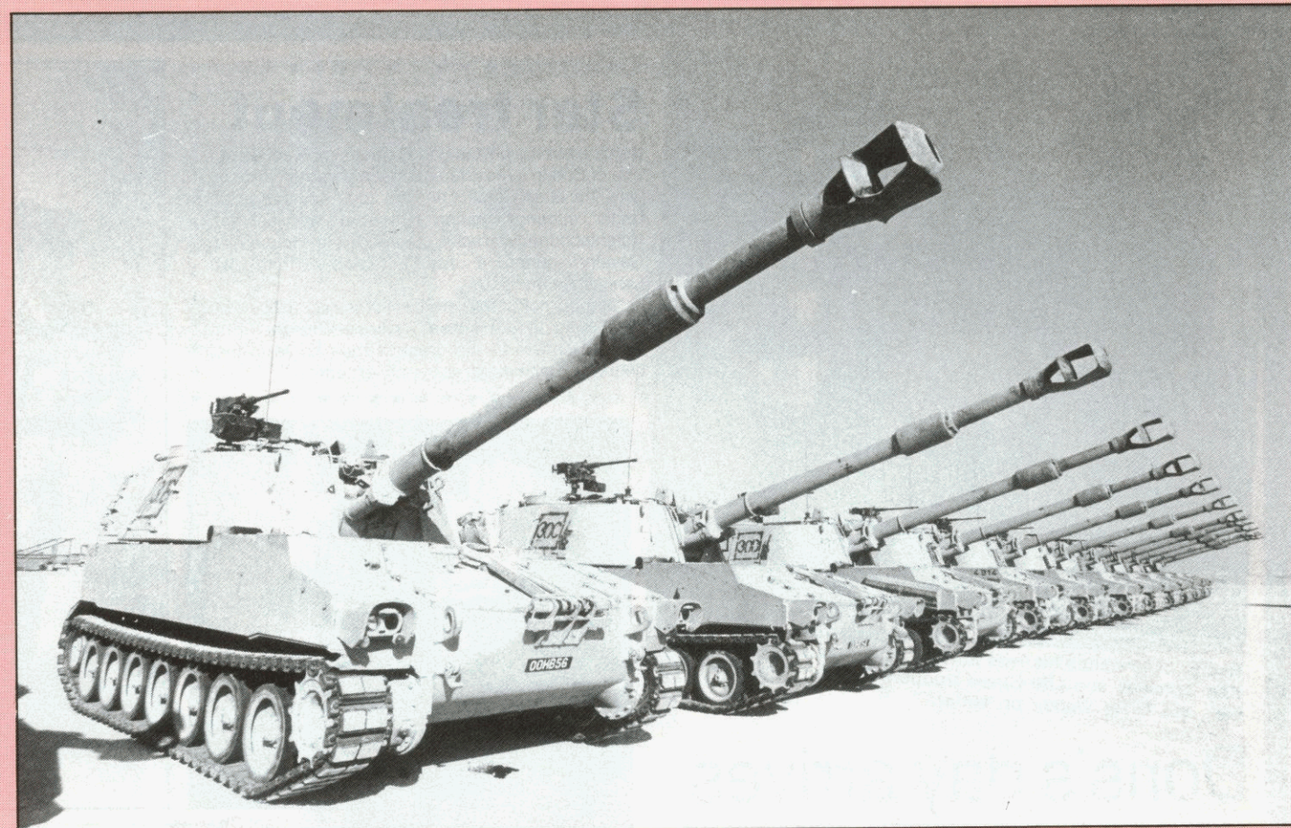
Still a force to be reckoned with after 25 years of service with the British Army, these M109A2 155mm self-propelled howitzers can lob a shell on to enemy positions more than 18,000 metres forward of their position
