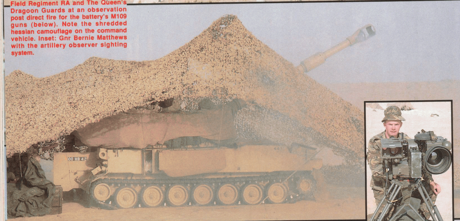
Still a force to be reckoned with after 25 years of service with the British Army, these M109A2 155mm self-propelled howitzers can lob a shell on to enemy positions more than 18,000 metres forward of their position
