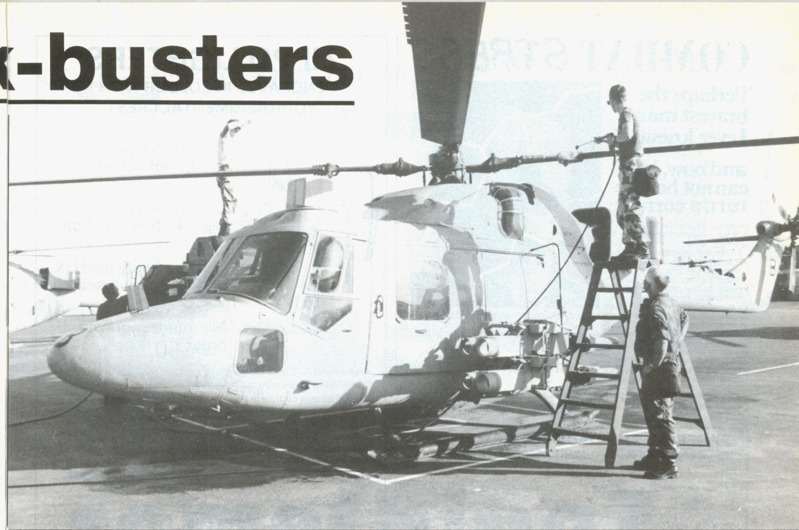
Army Air Corps groundcrew spray down a Lynx helicopter following a desert mission. Note the bulbous TOW missile sight above the windscreen
