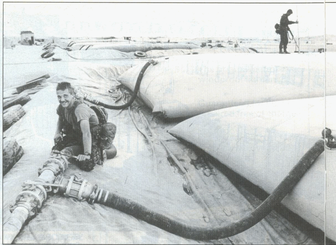
Pte "Sads" Saddington opens a valve on a portable fabric bulk storage fuel tank. In the background is LCpl Eric Sykes
