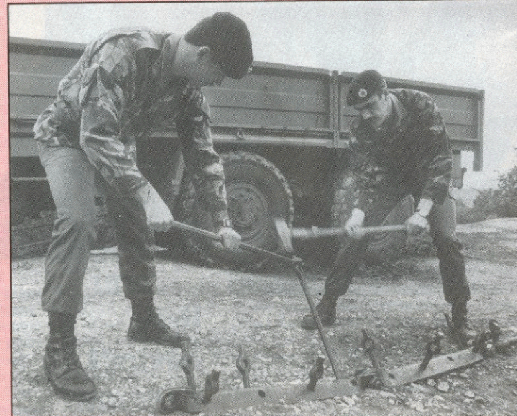
LCpl Geordie Bell (left) and LCpl Shaun Watson hammer in anchorage points to assist in a vehicle recovery
