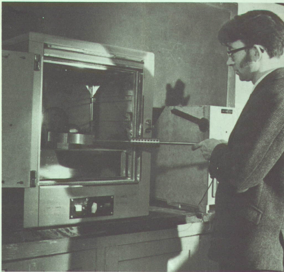
Left: Blow-forming the new zinc alloy Zam in an oven at 250 degrees Centigrade. The automobile industry has already shown great interest in it.
