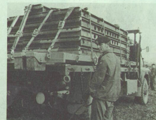
Above: Note hard rubber buffers under end of pallet on four-ton truck. The load is anchored to the ground and pulls off as the truck moves forward. Right: A 100-foot double-storey bridge erected during a test demonstration in Germany.
