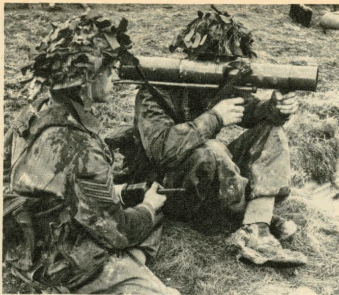
The Swedish Carl Gustav , an 84-mm anti-tank weapon with a "killing punch," is being considered as a replacement for the Infantry 3.5-inch rocket launcher.
