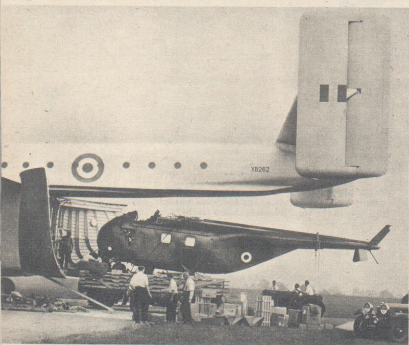
The Army's new transport plane can also be used as an ambulance. The main fuselage, shown here, holds 48 stretchers.
