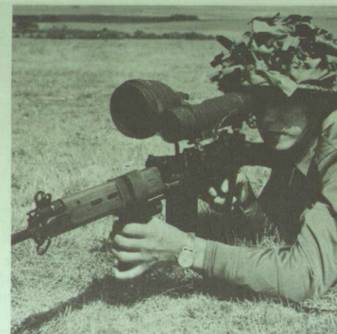
Left: The Dutch sniperscope on trial in 1961 was fitted with infra-red ray and could hit a target at 150 yards in the dark. Weight 15lbs.
