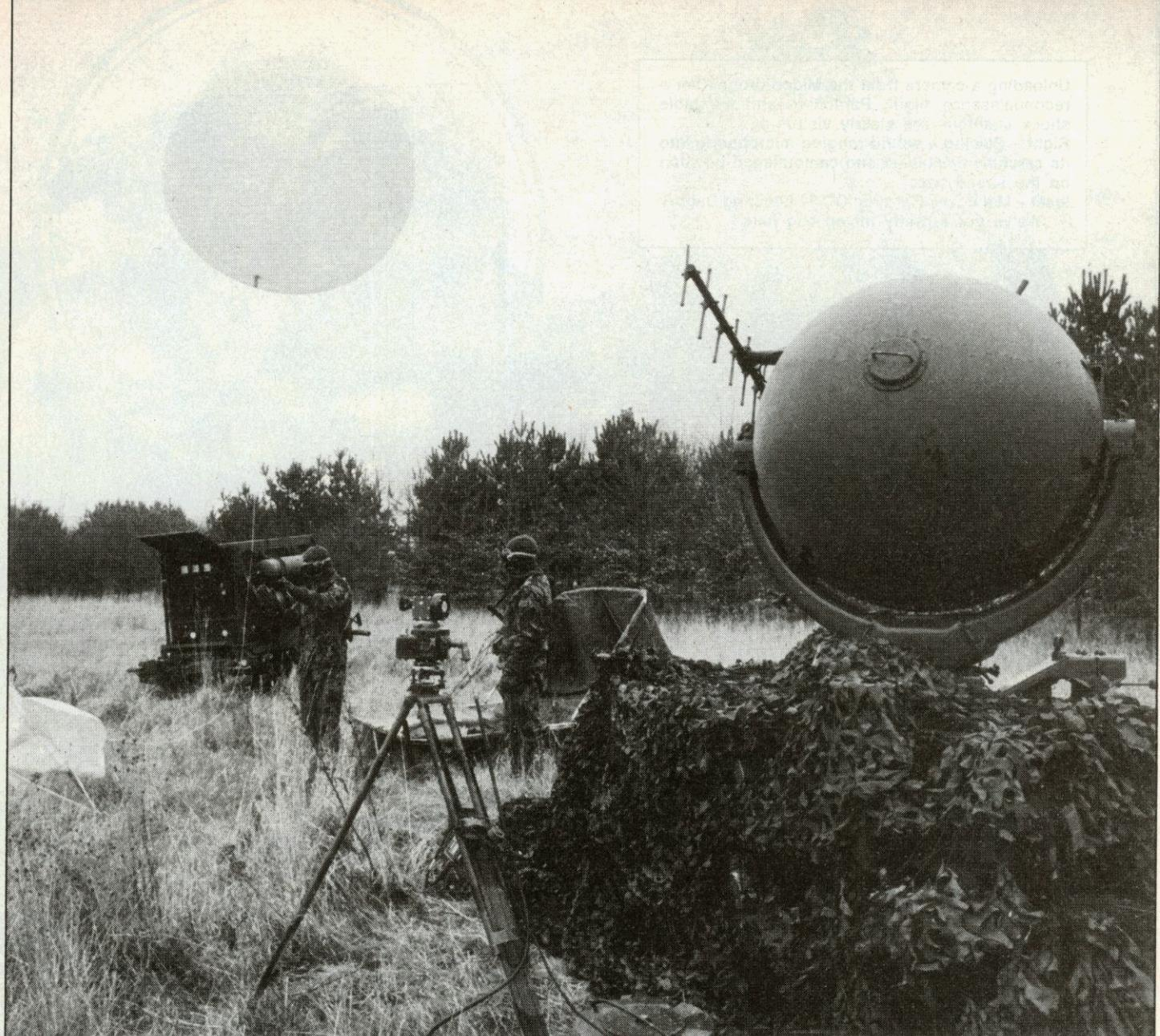
Men of the AMETS troop release a pilot balloon. They are wearing flash masks, gloves and goggles in case of malfunction with the hydrogen generator behind them. In the foreground is the radar tracking equipment
