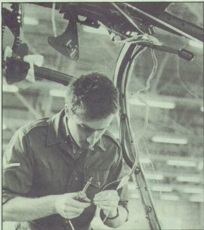
Lance Corporal Russel Cole joint soldering in the cabin of a Gazelle helicopter.
