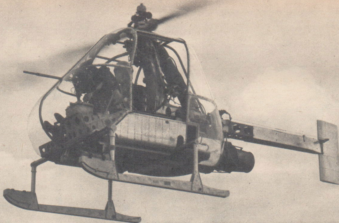
Designed especially for the Army: the Fairey ultra-light helicopter can be carried in a three-ton lorry. The "gun" pointing forward is the pressure head of the air speed indicator.
