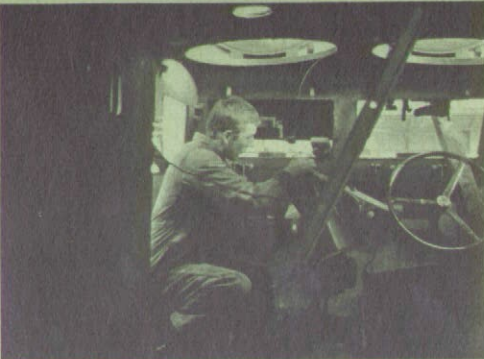
The vehicles' interiors were stripped out to take the new protective armour plating.
