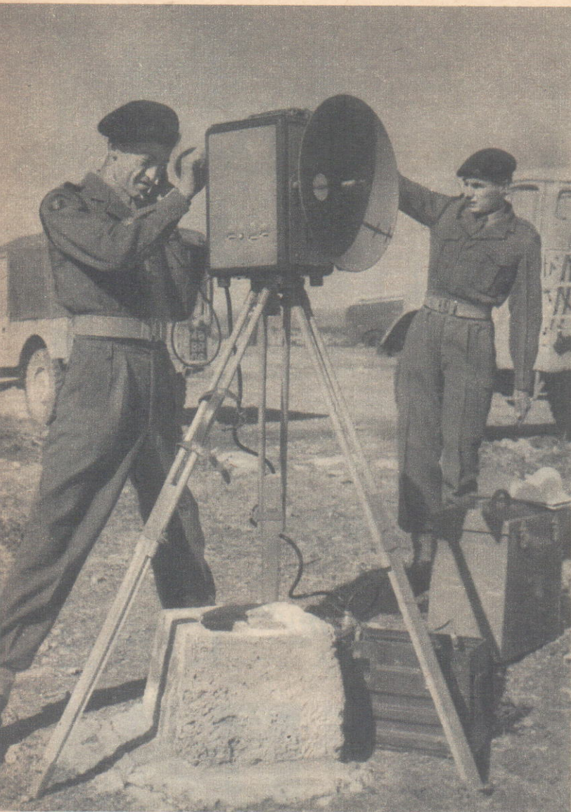
The Tellurometer at work with SSM J. D. Kennedy, Royal Engineers, at the controls. The instrument sends out radio signals along the line to be measured and is extremely accurate.
