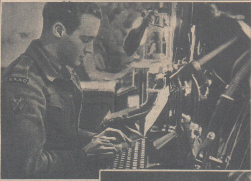
Private Michael Patton takes over the linotype from the German operator when important documents have to be set. Rhine Army's No. 1 Printing and Duplicating Unit tackles everything down to windscreen labels.
