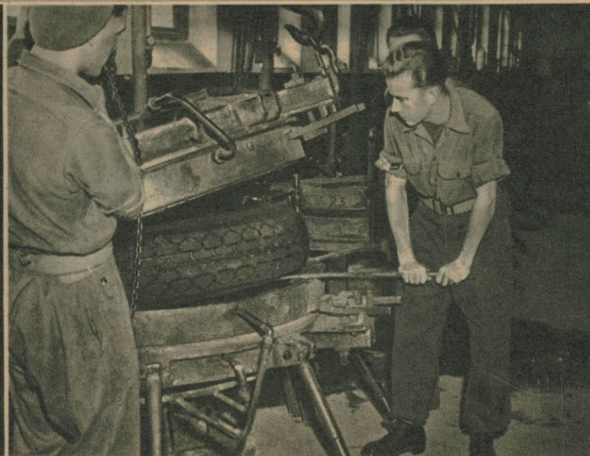
L/Cpl. W. S. Furber and Cpl. G. Hicks lever the retreaded tyre out of the steam press.
