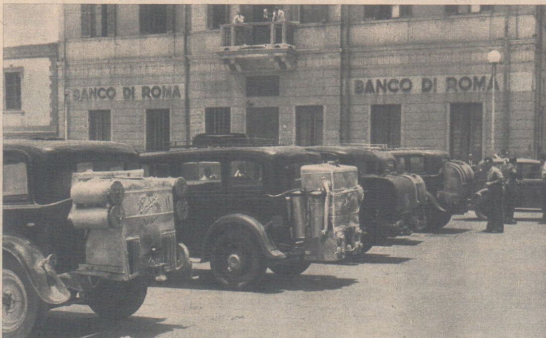
Left: One of the problems in colonies like Eritrea was to run transport without adequate fuel. Hence this row of cars with complicated gas engines at Asmara. Above: "Real money" in the eyes of the Ethiopians meant only Maria Theresa dollars (as minted in the 18th century). The British obliged by coining £3,000,000 worth.
