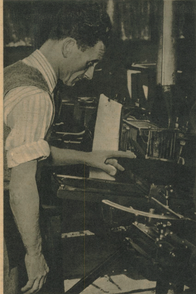
The beret goes under the "lawn mower" which trims away the surplus wool, gives it that close-cropped appearance.
