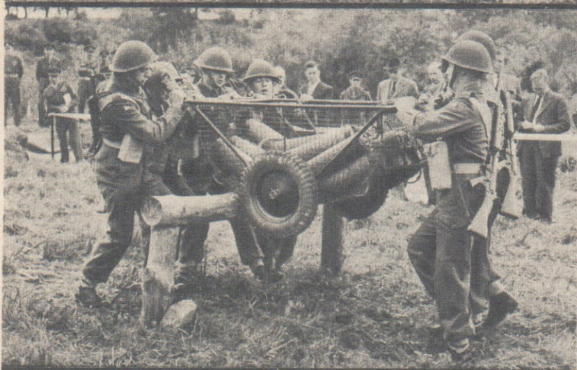
Guns on Salisbury Plain haul a universal load carrier containing 4.2-inch mortar ammunition over a two-foot high log.
