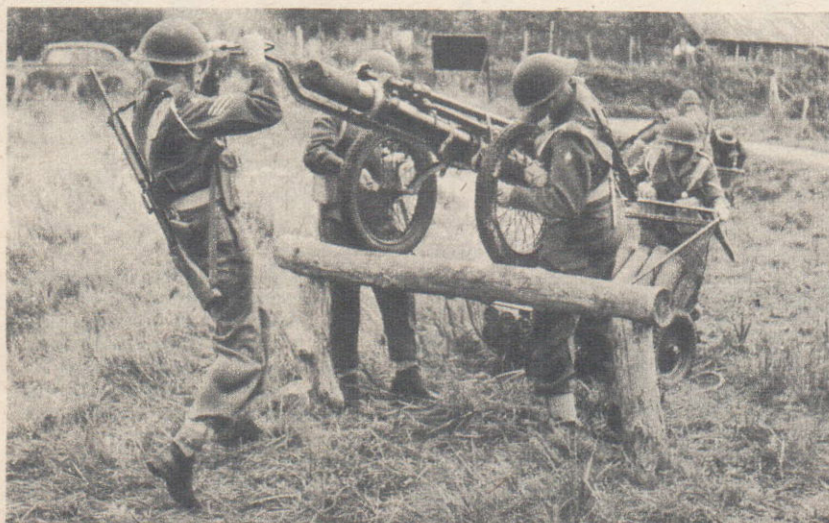
A 4.2-inch mortar on its trolley can easily be manhandled over obstacles. Normally, it is carried in a one-ton truck.
