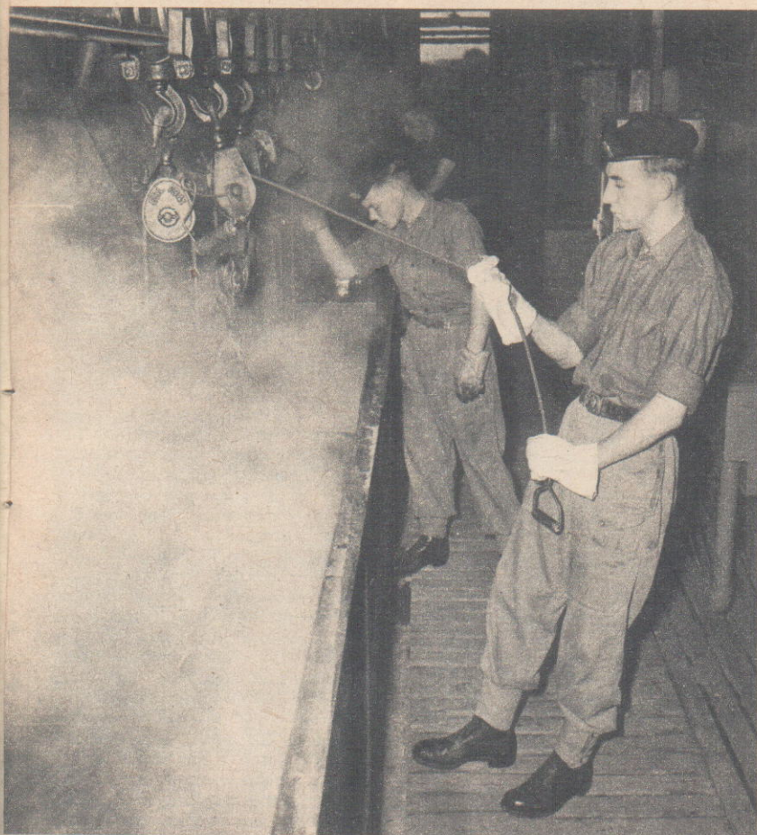
Left: Steaming alkali in the tank in the foreground removes grease from metal; water in the second tank removes the alkali.
