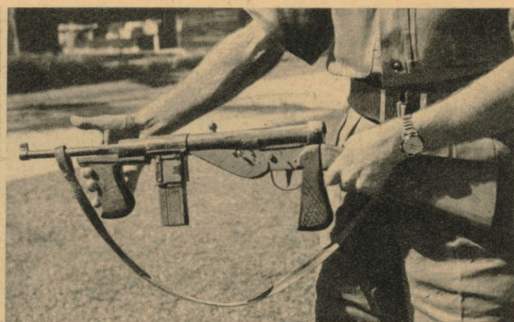
One you will not find in any gun-maker's catalogue. This bandit-made machine-carbine has parts from a Sten gun and a Thompson sub-machine-gun and a barrel from a No. 1 rifle. It fires .300 ammunition, is automatic only, and reasonably accurate up to 30 yards.
