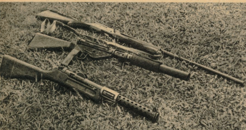
Close-up of three of the less well-known weapons in use in Malaya: a Browning automatic shot-gun (top), Sten gun with silencer (centre) and Lanchester 9 millimetre machine-carbine, which is used principally by the Royal Navy.
