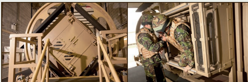
Roll-over: Simulators allow vehicle crews to practise escape methods that could be used in theatre
