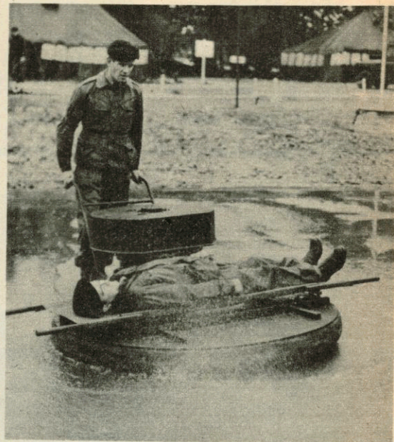
One man can operate the new Hoversled which rides over a cushion of air produced by an electric motor and can carry two casualties over the roughest ground without rocking them. It can be towed, patients aboard, behind a vehicle.
