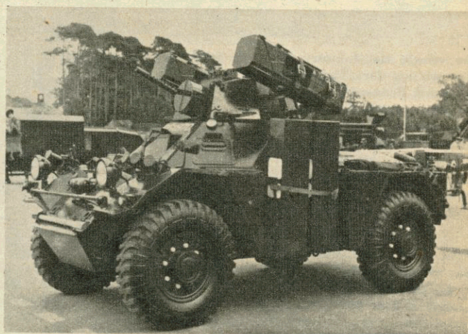
Left: Peeping Tom , the tiny, radio-controlled drone which spies out enemy positions and returns to base by parachute. Above: A Ferret scout car fitted with two Vigilant wire-guided anti-tank missiles.
