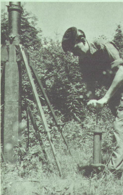
Above: Blow-up. Not dynamite but pneumatically operated aerial mast. It is worked here by hand but normally the vehicle's compressor is used.
