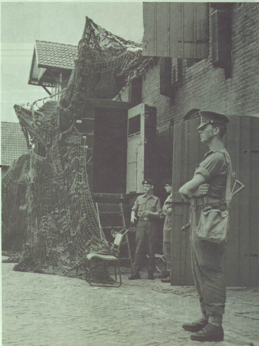
Above: Blow-up. Not dynamite but pneumatically operated aerial mast. It is worked here by hand but normally the vehicle's compressor is used.
