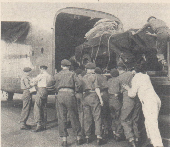
On rollers, the load slips easily from a truck into the aircraft. Right: The parcelled jeep swings to the ground.
