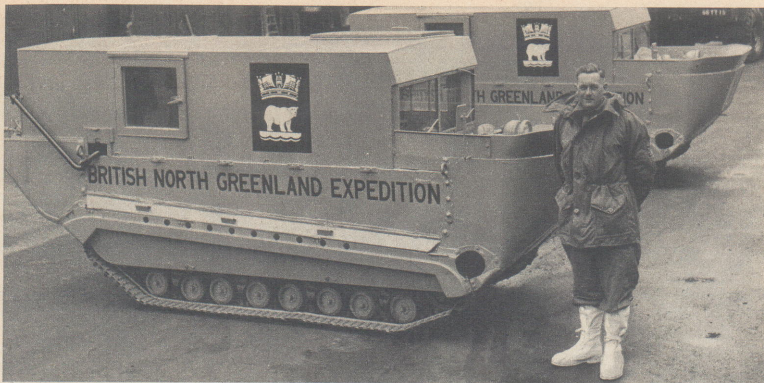
Two of the modified Weasels, with their insulated cabins. They are painted orange, in order that they may easily be seen in the snow.
