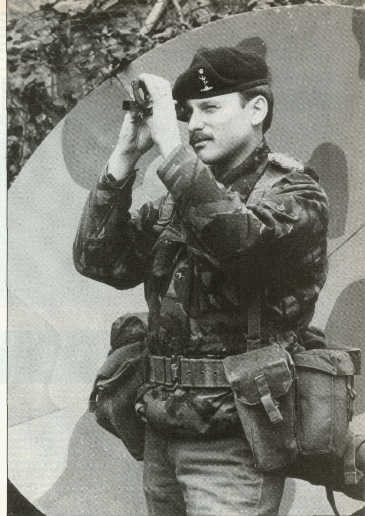
Cpl Keith Barker checks out the elevation angle of the satellite using an inclinometer
