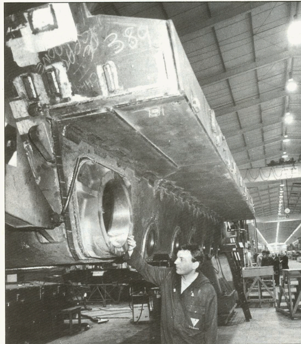
First picture of the new tank in the early stages of production. A Vickers employee checks the machining of the hull of the first prototype main battle tank
