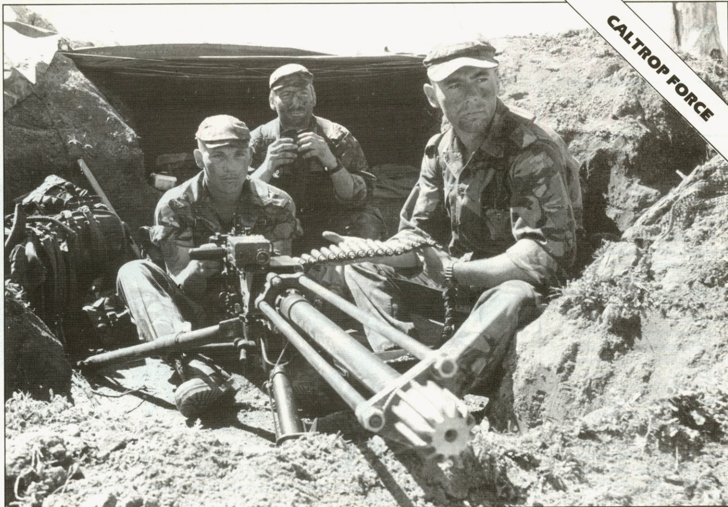
A machine-gun detachment of 1 Para dug in with a .50 calibre Browning. The MG platoon had dropped with GPMGs (7.62) but took over the Brownings when they were airlanded and handed over their original weapons to the rifle companies. Gun and tripod weigh 120lbs. The rods and fluted muzzle shown here round the barrel are fitted when firing blank ammunition. Left to right are Pte Fitz Fitzwater, Cpl Clive Mills and Pte Steve Imrie
