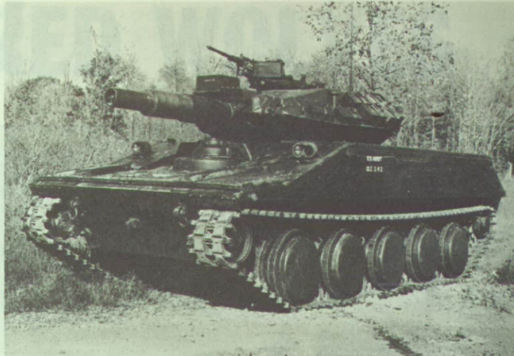
Above: The American General Sheridan tank can fire the Shillelagh missile and is air-portable. It is a recon tank for armour and Infantry.
