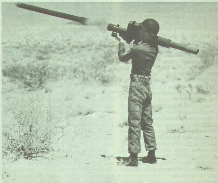
Redeye, the world's smallest guided missile, is fired from a shoulder launcher (below). At a safe distance its motor fires, driving it on to target.
