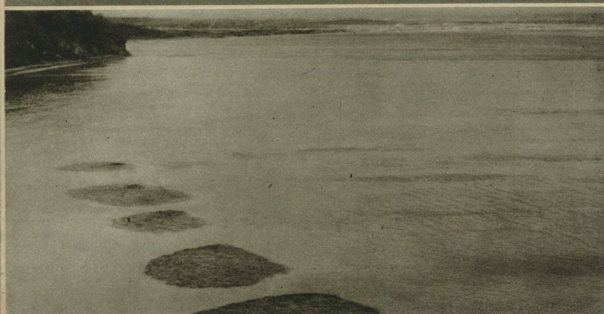
Above : oil projected into the sea from pipe lines to form a continuous line ready for ignition. Below (left) : the oil is ignited ; (centre) the sea is on fire ; (right) finger of flame used on ships against low-flying aircraft.
