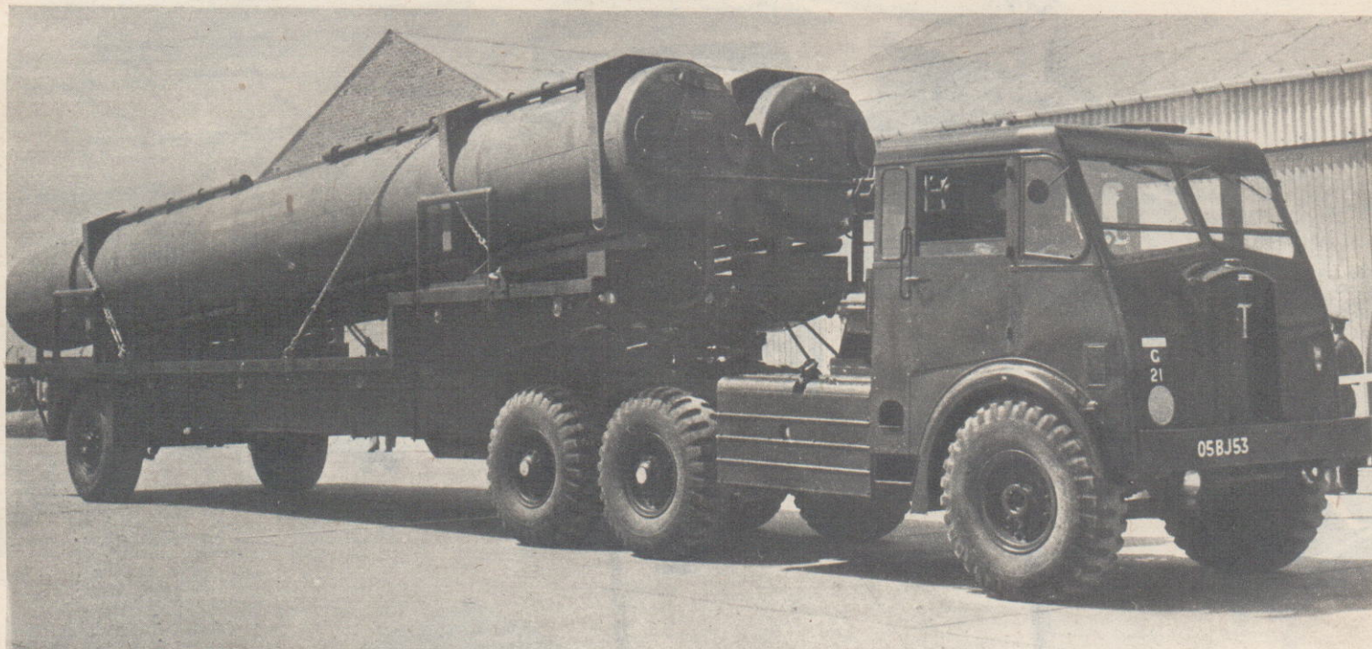
This load does not contain milk, molasses or diesel oil—just two Corporals, hermetically sealed. Below: The launcher, on which the missile rests before take-off, under tow.
