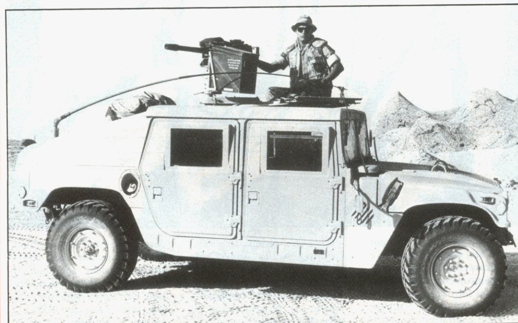
Hummvee armament carrier version fitted with Mk 19 automatic grenade launcher
