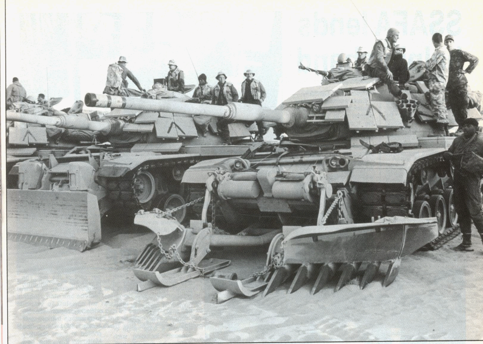
US Marine Corps M60A1 main battle tanks and crews await the arrival of tank transporters to move them to the front line. Note the mine clearance plough fitted to the front of the vehicle and the explosive-reactive armour fitted around the turret
