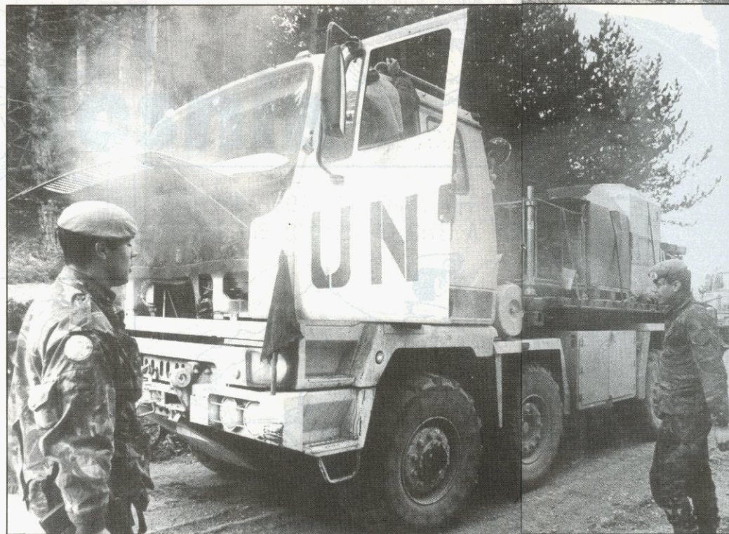
Smoke pours from the engine compartment of DROPS vehicle "Zero five". A broken coolant hose was hastily patched up by LCpl Tony Sharp of the REME
