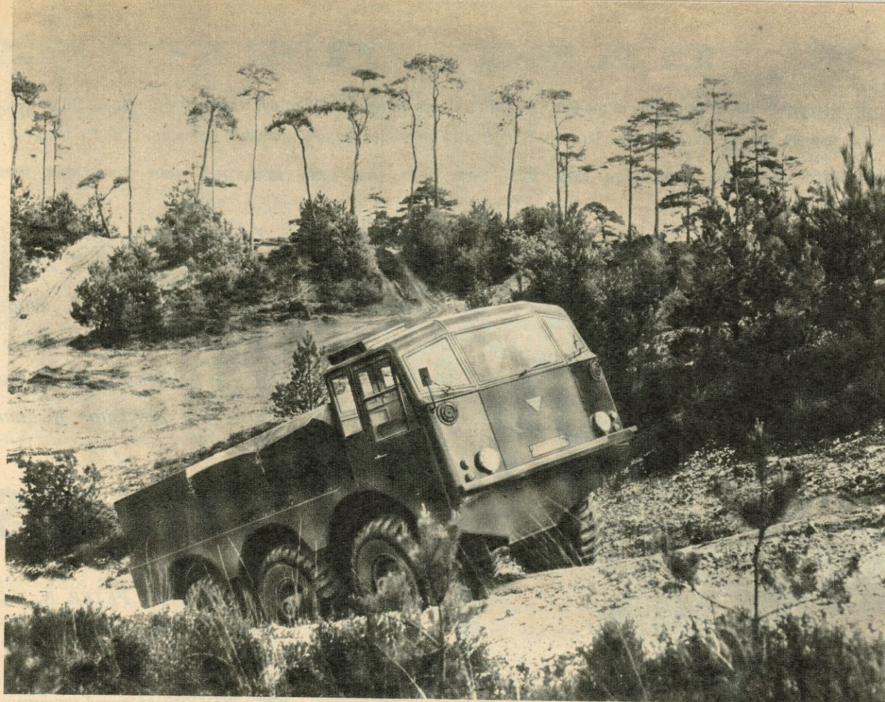
The Stalwart grinds up a one-in-three hill on trials. It can also cross a five-ft. wide trench.
