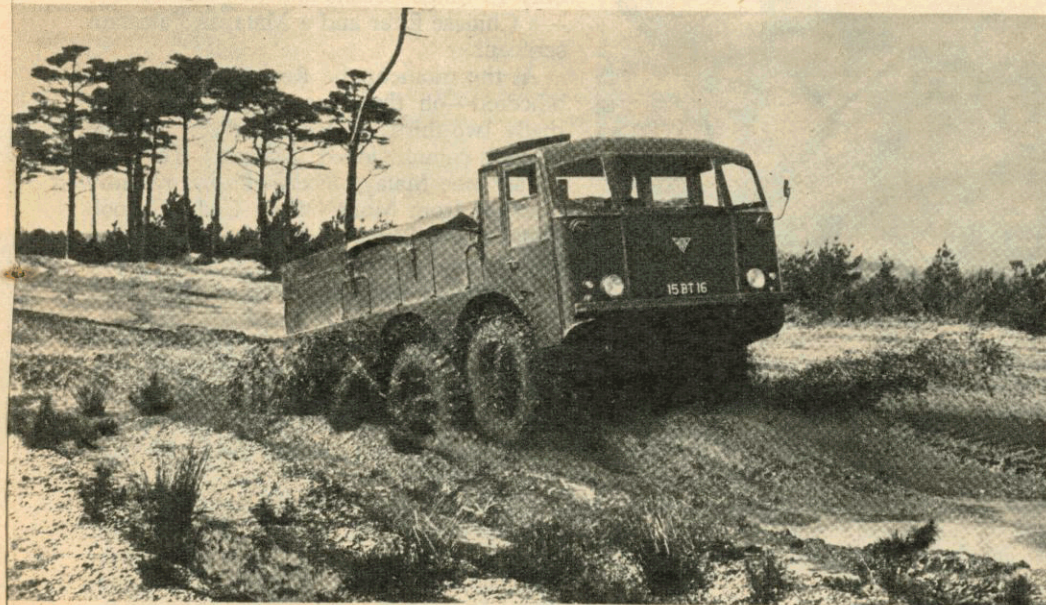
Above: Note the size of the six wheels suspended on an articulated chassis. Left: Ploughing through deep water and mud.
