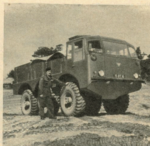
Above: Note the size of the six wheels suspended on an articulated chassis. Left: Ploughing through deep water and mud.
