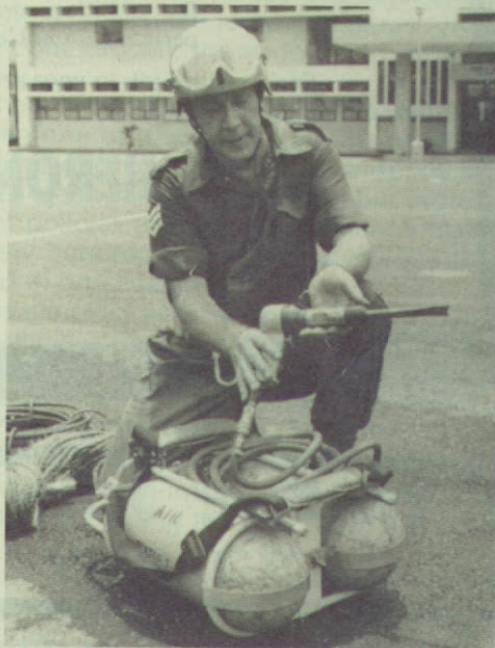
The ripper gun, with its compressed air drive, can tear away wreckage at speed.
