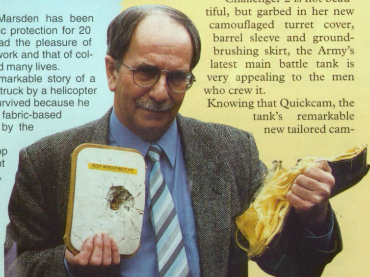
Tested to destruction. Ballistic protection expert Tony Marsden with the aramid fabric and ceramic products which are giving British soldiers ever more protection from bullets and shrapnel
