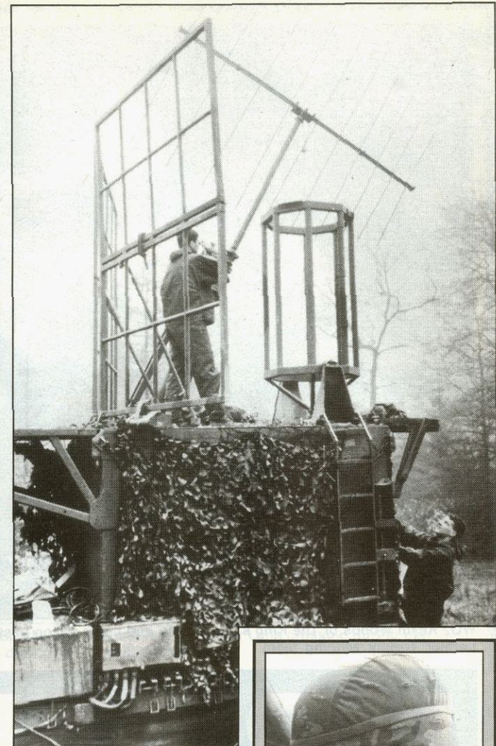
Above - Bromure antenna is raised into position. The window-like frame on the left directs the jamming signal with devastating accuracy
