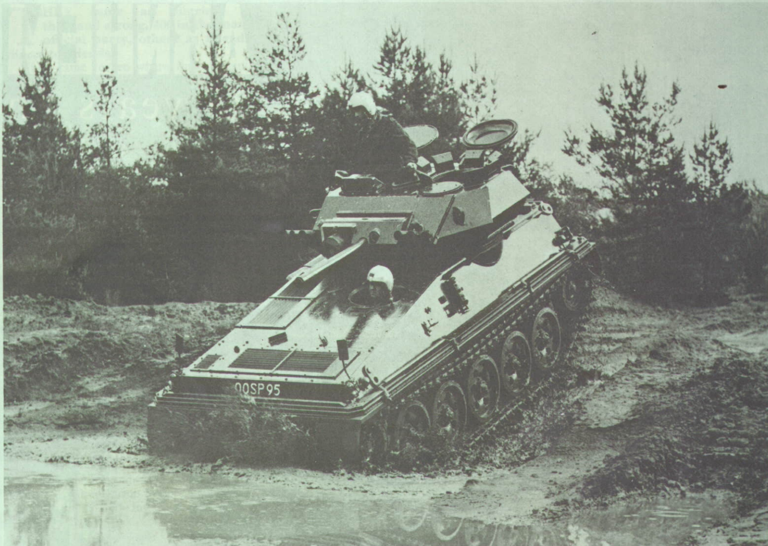
A built-in screen enables Scorpion to swim without further preparation. Its concertina folds can be clearly seen in these two pictures.
