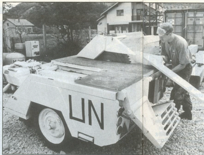
LCpl Don Ridley checks out a trailer-mounted wood saw which has been taken into service by 1st Field Squadron
