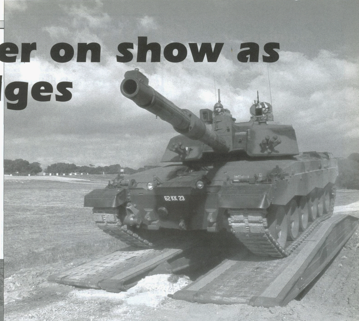
A potent combination: Challenger 2 rumbles over the Royal Engineers' versatile new close support bridging system during a confidence-building demonstration at the RAC Centre range
