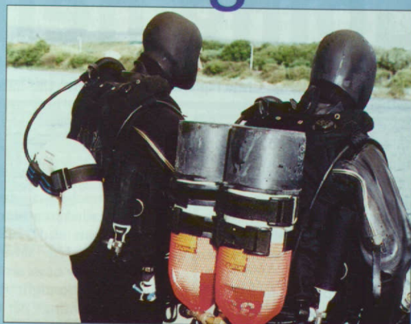
Where's my donut? The small, nine-litre, toroidal vessel, left, as it would be used by a diver pictured for comparison alongside conventional cylindrical compressed-air containers
