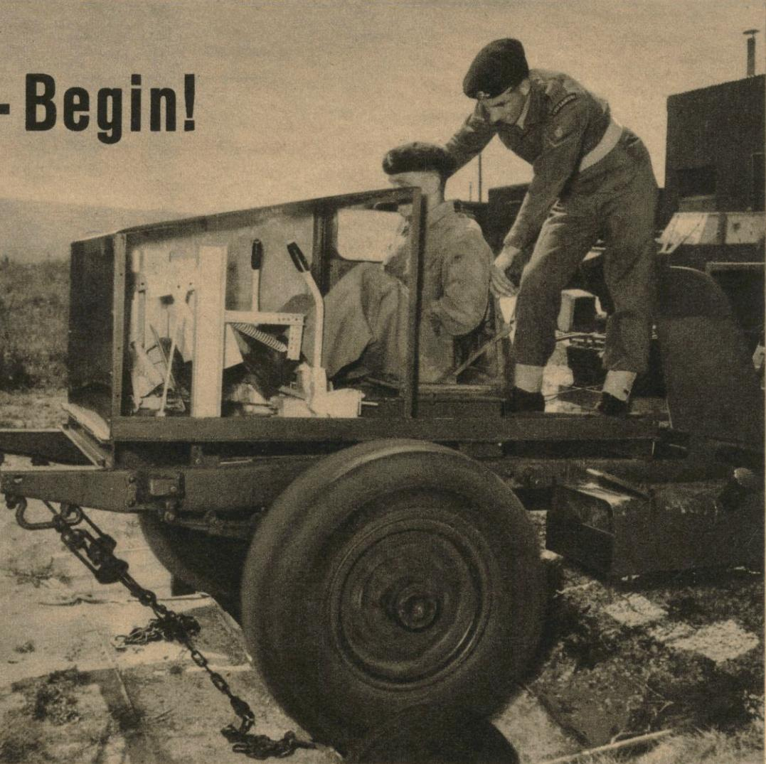
The wheels go round, but the vehicle stays still. This curious hybrid is a Bedford chassis with tank controls fitted to it.
