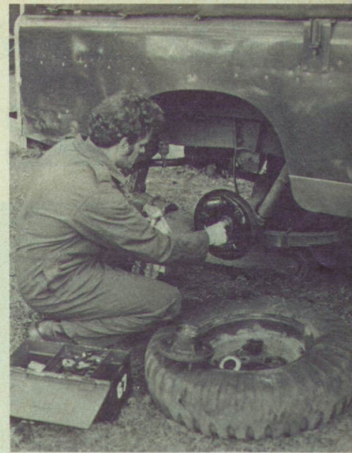
Above: A REME mechanic carries out a quick changeover of the oil seal on a Land-Rover.
