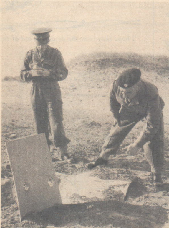
Cardboard targets are used to test impact fuzes on the ranges at Pendine. If the round passes through, leaving a neat hole (above) the fuze is faulty. If the targets are damaged like those at right, the fuze is correctly made.
