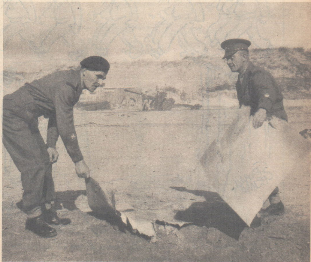
Cardboard targets are used to test impact fuzes on the ranges at Pendine. If the round passes through, leaving a neat hole (above) the fuze is faulty. If the targets are damaged like those at right, the fuze is correctly made.
