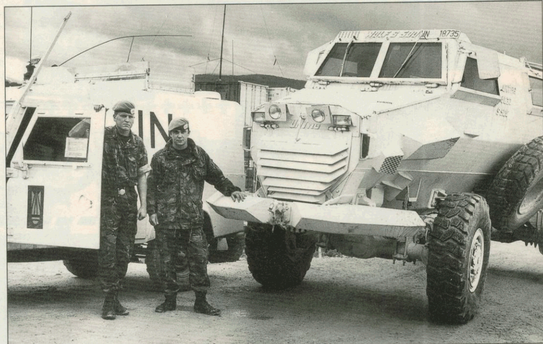
Spr Des Clulow and Wayne Bye from Wimbish-based 33 Engineer Regiment (EOD) encounter a strange-looking United Nations vehicle. The Wolf is designed to withstand a mine explosion. Its double-skinned body is filled with water to deaden the shock wave, while the angled hull deflects the effect of blast
