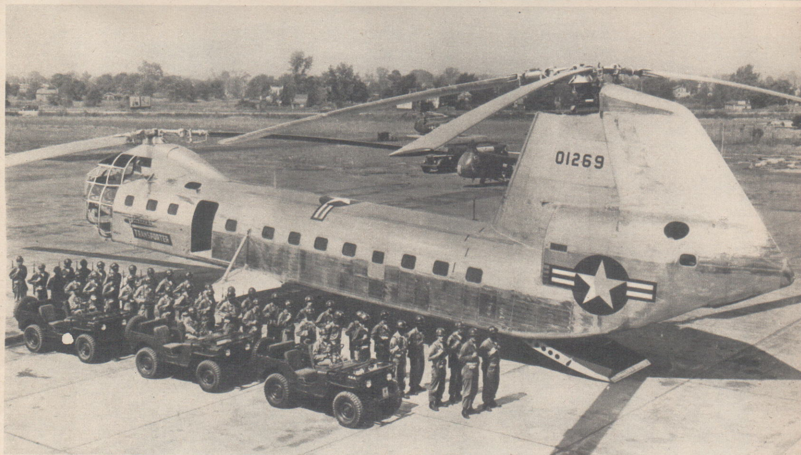
This American tandem helicopter will carry 40 men or three jeeps. A British firm is contemplating a helicopter to lift 450 troops or a 45-ton tank
