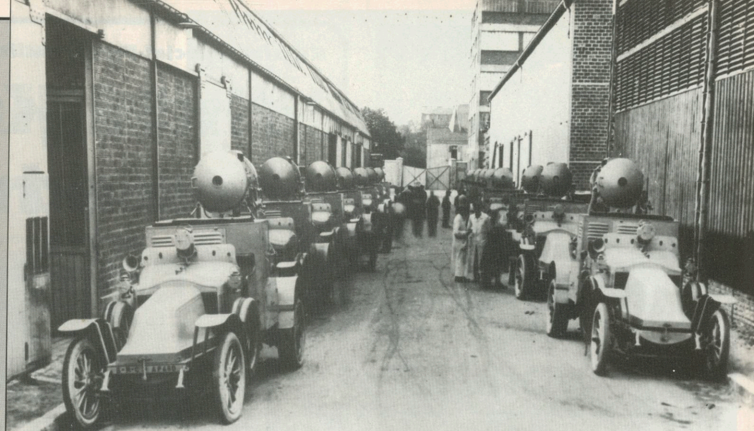
Searchlight cars at the Renault factory at Billancourt (Seine). This photograph was taken in 1917 but Renault had been fitting searchlight and signal lights for military purposes from as early as 1900
