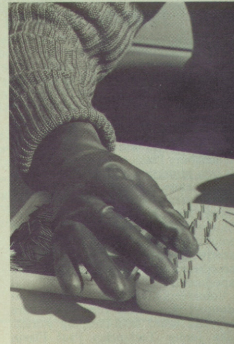
Above: Testing the speed of a man's reflexes. He follows a light round with a probe—when he catches it up it bleeps.
