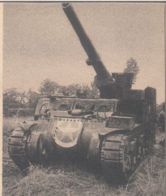
Left: This American tank destroyer, mounted on a Sherman chassis, proved its worth in Normandy. Right: "King Kong," the American Army's 155 mm gun on a Sherman chassis, which was the heaviest self-propelled gun to go into action.
