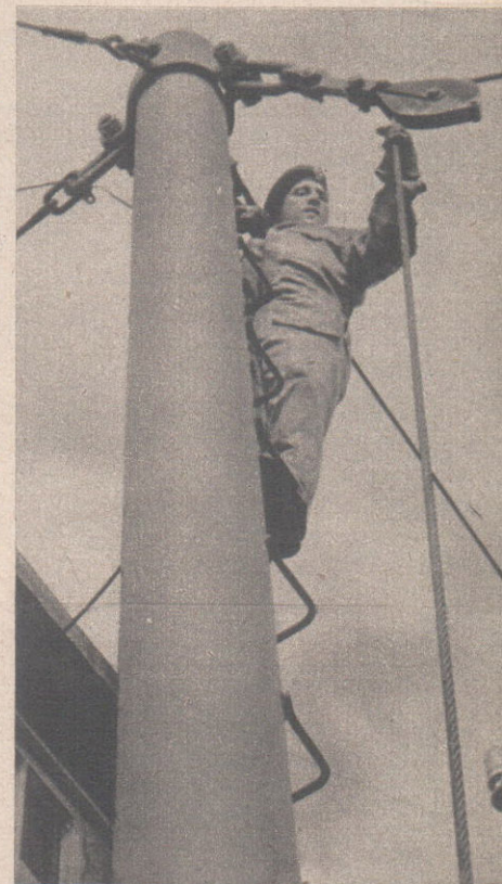
Sapper R. Robinson shins up the Samson post to clear a fouled block.
