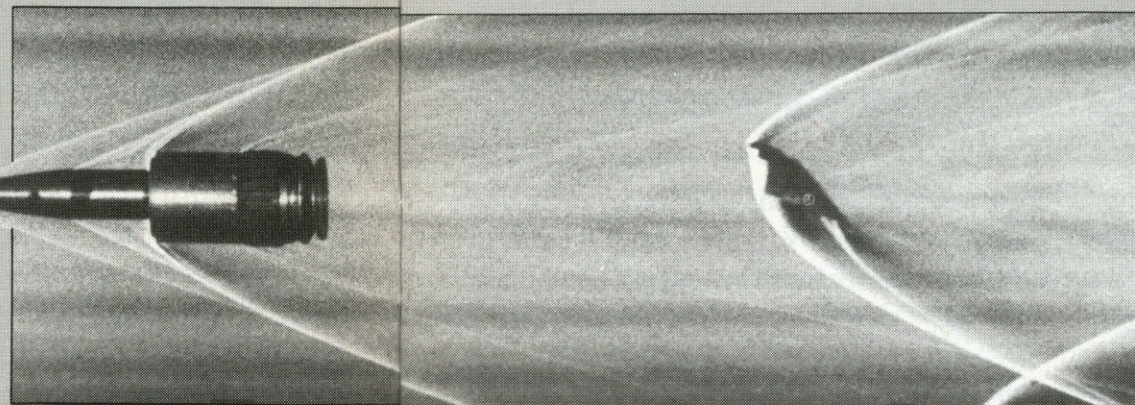
An example of the high speed photographic work done at Pendine. It shows a 30mm Rarden APDS shell in flight
