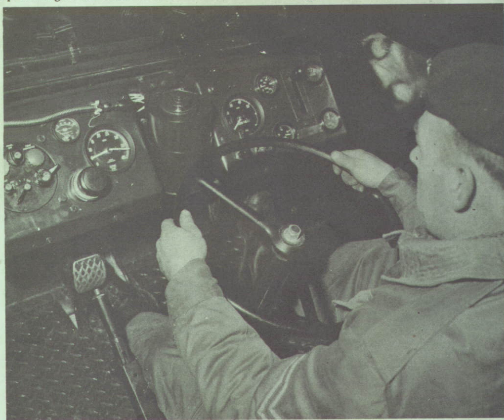
Cpl H Mudge RASC at the wheel of his Stalwart . The driving position is in the middle of the cab.
