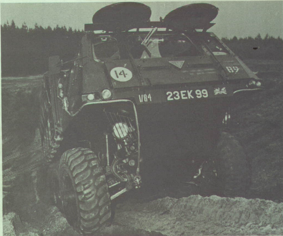
Up a sharp incline on the RASC test track in Germany, a Stalwart displays its boat-shaped belly.
