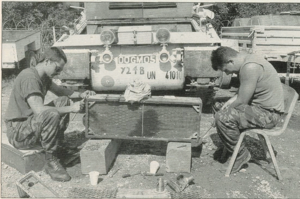
Cfn Kevin Irvine and Cpl Gary Lewis, serving with the QRL's REME LAD, repair a Scimitar radiator
