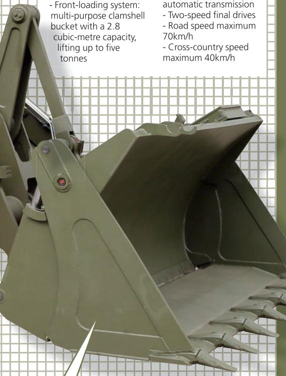
**Greater grip:** The multi-purpose bucket and excavator arm can fill craters, dig and construct earthworks, mechanically place obstacles and doze over and level surfaces, giving it the ability to bridge natural or man-made voids. Terrier can also grip and lift objects, breach earthworks and remove obstructions such as barricades. With its rock hammer it can destroy and disrupt concrete obstacles.
