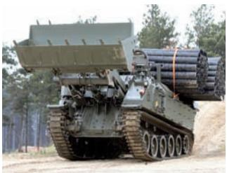
**Top marks:** An integrated lane-marking system allows the Terrier to highlight safe routes to vehicles behind it.
