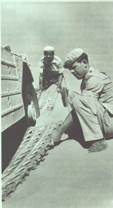
Below: "Unsticking" a Ferret with pierced steel planking which is carried clamped to vehicle.
