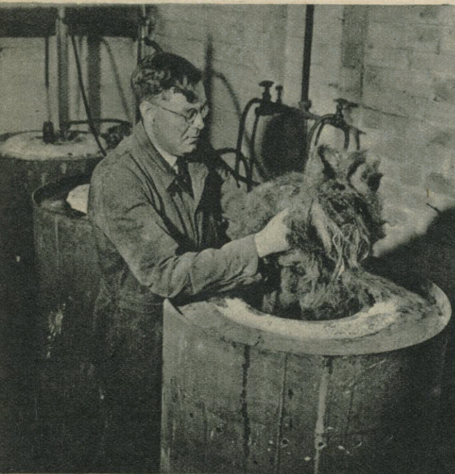
7 More caustic soda is added. The hair, which is getting pretty weary by now, gives up the struggle and cystine separates out.
