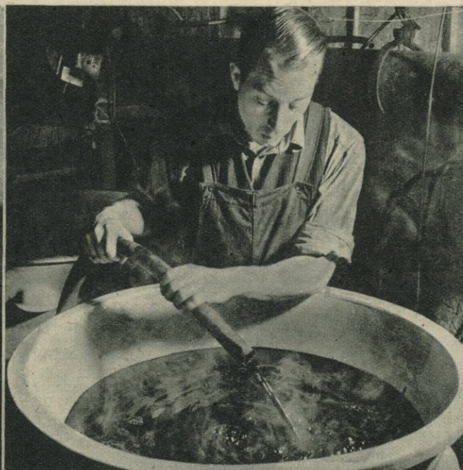
8 Pure cystine separates as a brilliant white powder which is filtered and dried. Charcoal is used in the cleaning process.
