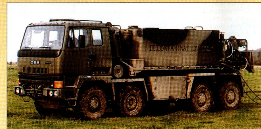
Spray it: Multi-Purpose Decontamination Equipment provides one of the three main capabilities of the Joint NBC Regiment. The Karcher kit was bought for use during the Gulf War and constructed on DROPS flatbeds. The disinfecting gear will be used primarily to decontaminate high-value assets such as command and control and the Fuchs vehicles
